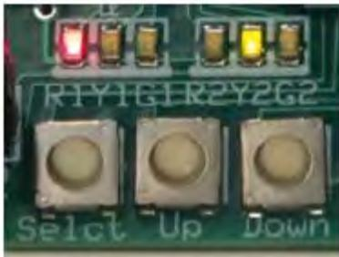
Figure 2 Decoder buttons and LED's
