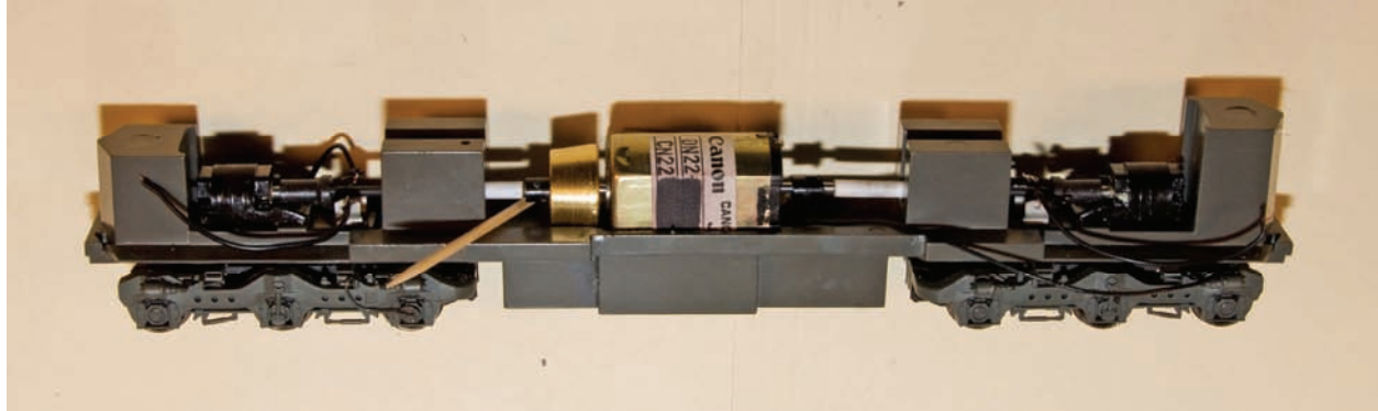
Athearn SP SD50 re-motored with a Canon DN-22
