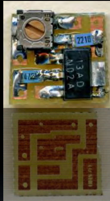
Neg. Voltage Regulator for Engines 7/16" x 5/8" LM337 SOT-223 Case
