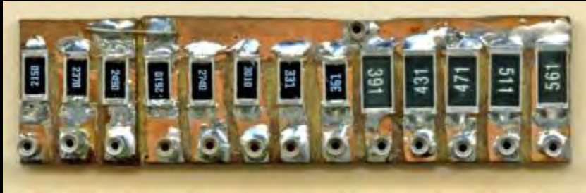
215Ω to 561Ω Test Board
